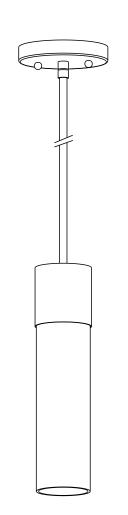
Canopy **Brushed Nickel** Brushed nickel (3X12"+1X6") Rod Max. 42" (3X12"+6") Die-Cast metal housing **Brushed Nickel** Medium Base 1X60W A15 or T10 White Opal hand blown Glass
